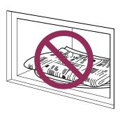
**Do not** try to melt paraffin wax in the oven. Paraffin wax will not melt in a microwave oven because it allows microwaves to pass through it.
